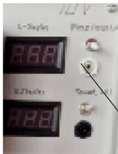
Switch is on top position: Voltage from MA, down position: Voltage from the safety plug (IW 64)
