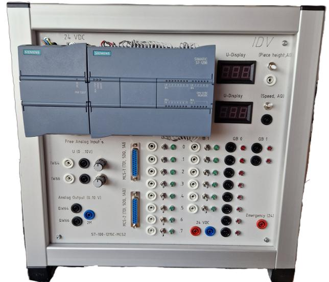
Digital Voltage Display is direct conneted with SUB-D 1 to measure the height of the workpieces, if you connect MCS-520 there, or to show the voltage on the safety plug (Switch).
